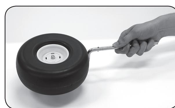
Slide wheel then hubcap onto axle.
