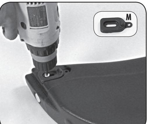
Install door latch using number of screws required as shown.
