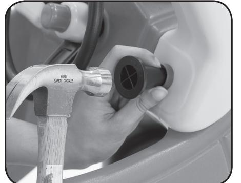
Place axle cap tool over ignition base and hammer.
