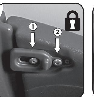
Latch in permanent "locked" position; install (2) 1/2" (1,27) screw.
