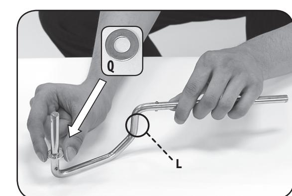
Slide washer onto the short end of the LEFT front axle marked "L".
